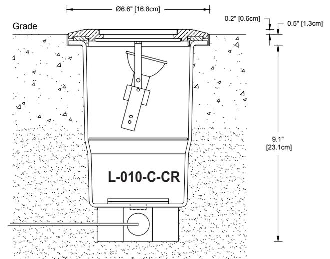
Fixtures supplied with 15 ft. [4.5 m] type SJOOW cord for remote connectors.
