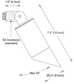
This directional downlight is certified by DarkSky International when mounted on a VERTICAL surface and aimed downward. This fixture will not work nor be DarkSky compliant if mounted to a horizontal surface such as the ground or ceiling.
