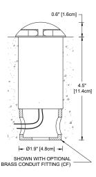
Fixture can be stabilized using conduit & fittings or a pipe nipple attached to a plate on the ground and threaded into the bottom hole of the CF or the PVC Cap in the CFK.
