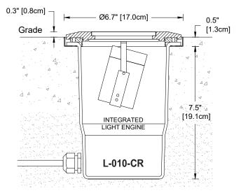
Fixtures supplied with 10 ft. [3 m] type SJOOW cord for remote connectors.
