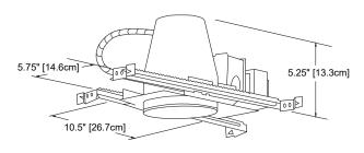
Ceiling Opening: Ø4-3/8" Max Ceiling Thickness: 1"
