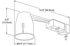
Ceiling Opening: Ø4-1/8" Max Ceiling Thickness: 1-1/4"
